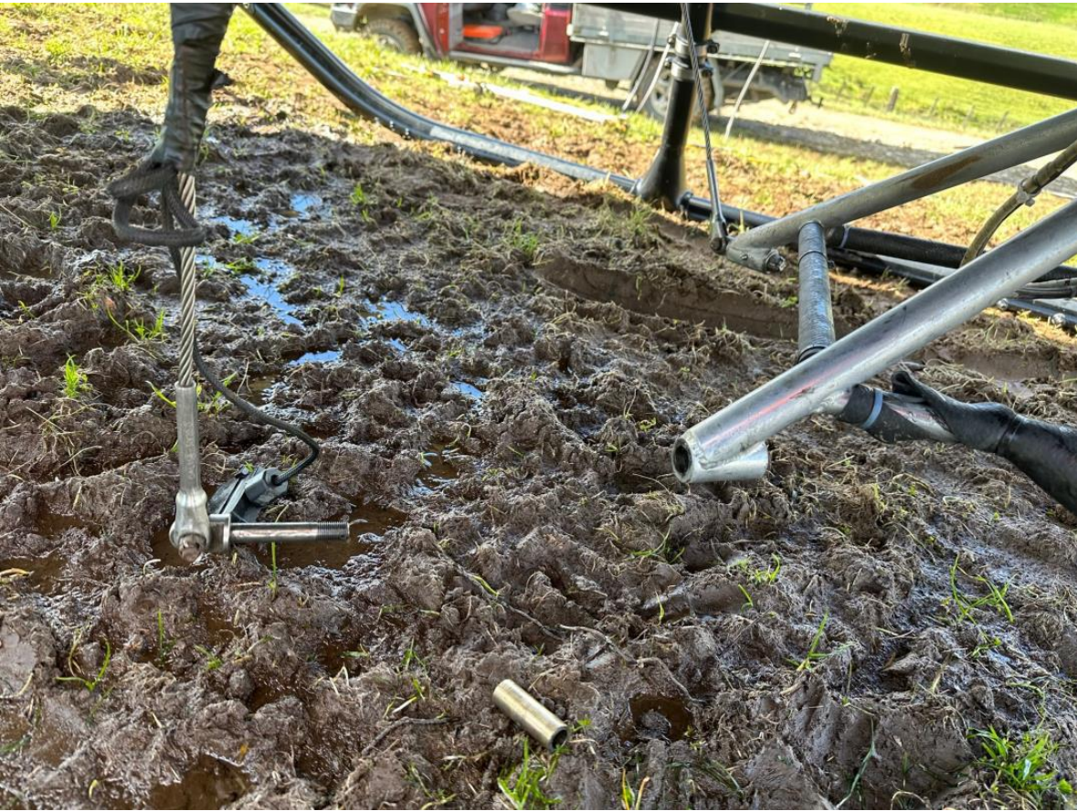
Figure 1 Hook Swing Frame attachment failed in flight
