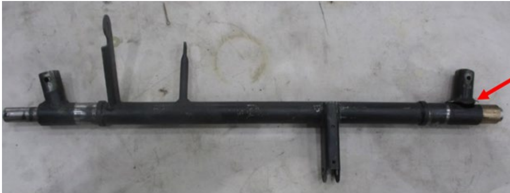
Figure 1 – Rudder pedal bar failure location
