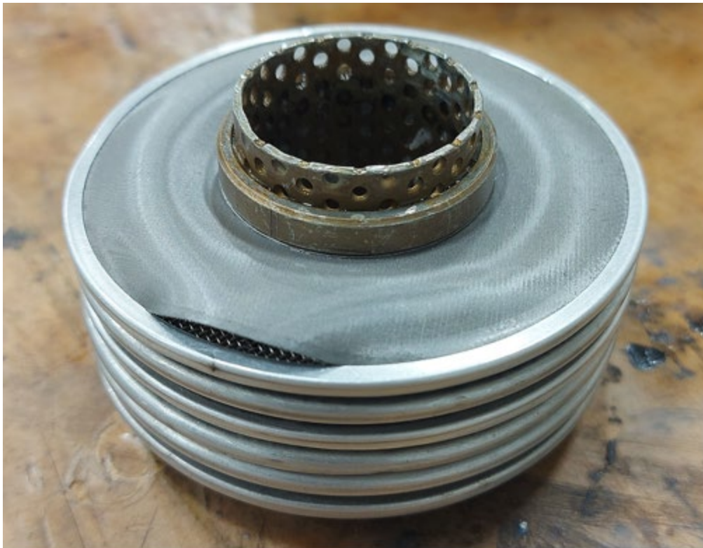
Figure 1 – Bulged filter disc due to the fuel flowing in the opposite direction than designed
