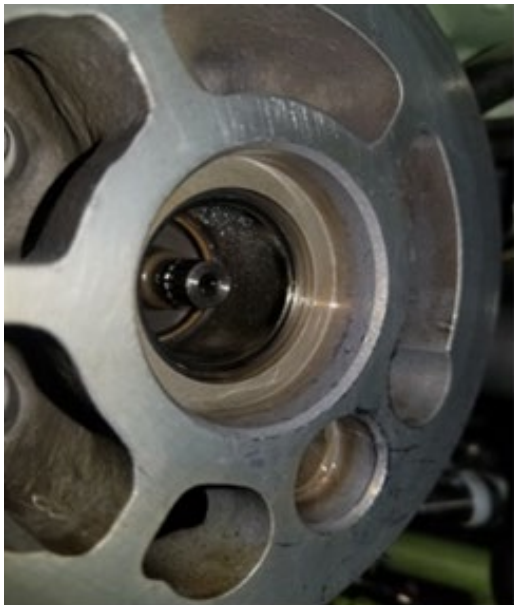
Photo 2 – Fuel pump drive spline
