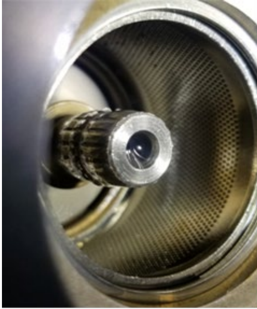
Photo 3 – Fuel pump drive spline close-up view
