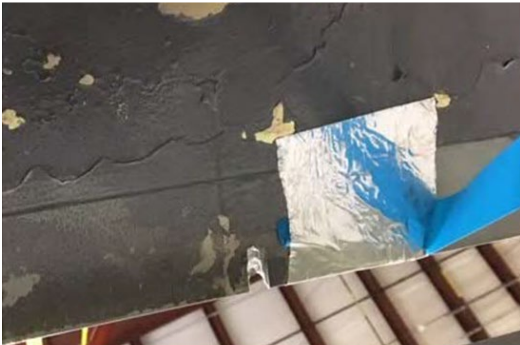
Figure 2: Close-up of slat damage
