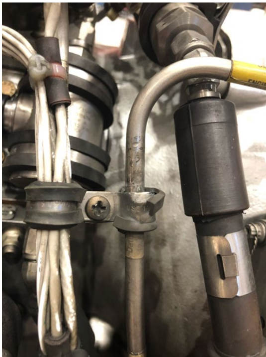
Picture 1 – Damaged clamp attached to tube on the engine
