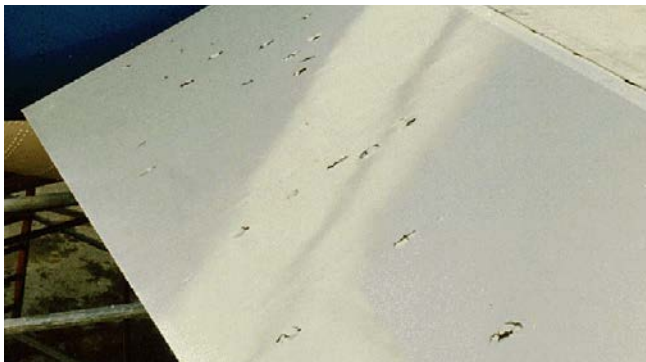
Dents and Punctures on Boeing 757 Inboard Aft Flap (thin skin of composite sandwich)
