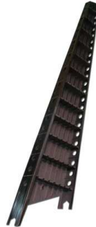
Vertical fin structure : VaRTM process
