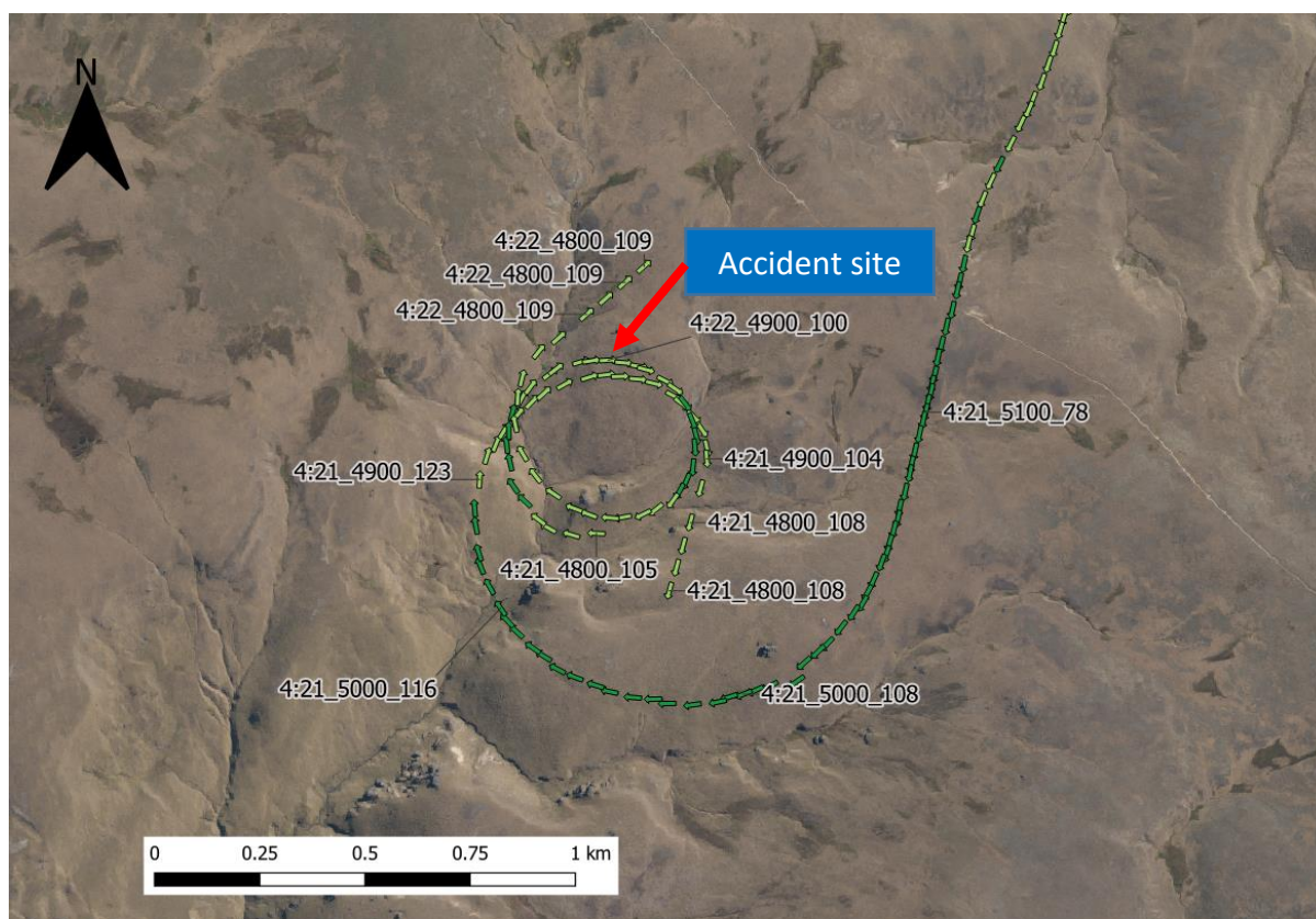
Figure 6 MLAT flight track data; time (UTC) altitude (AMSL) groundspeed (Kts). (Straight lines of arrows indicates predicted flight path after a loss of signal)
