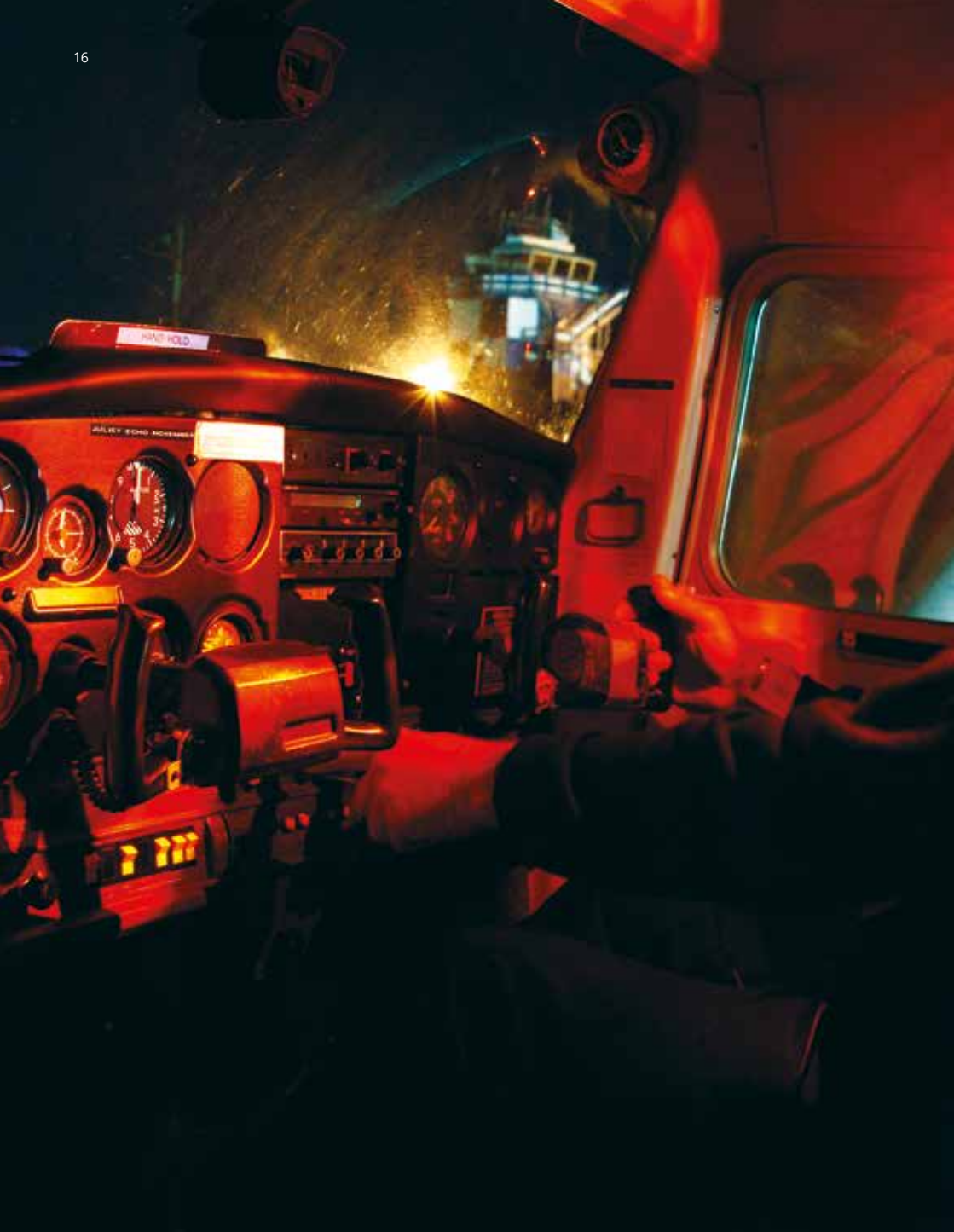
A headband torch with red filter being used for cockpit lighting.
