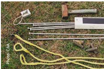
Figure 5 - Two types of pickets most commonly used for grass areas.
