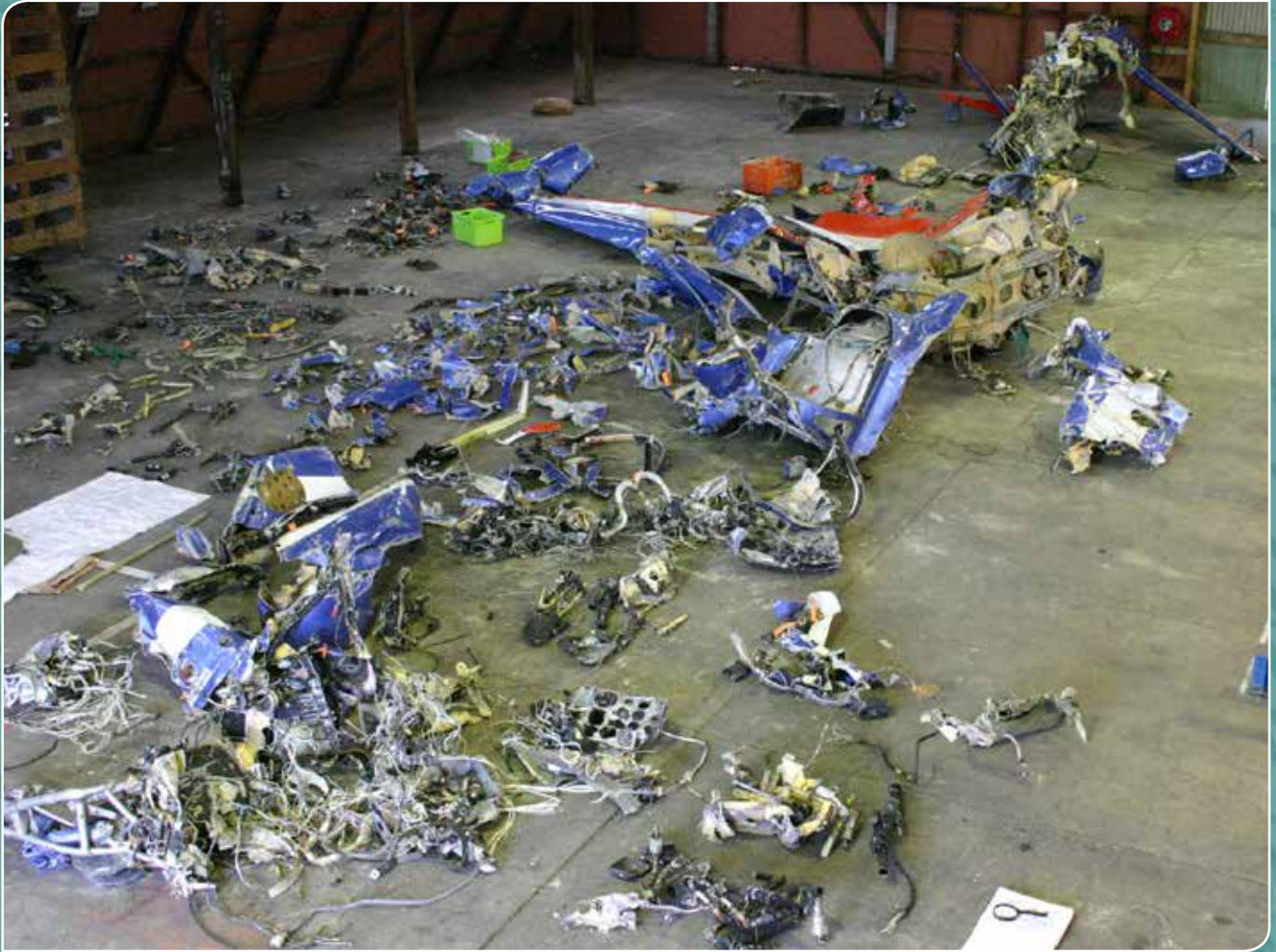
Once recovered from the water, Alan Moselen had to painstakingly lay out the wreckage of the aircraft to reflect its actual configuration, to eliminate or confirm the possibility of a mechanical problem.
