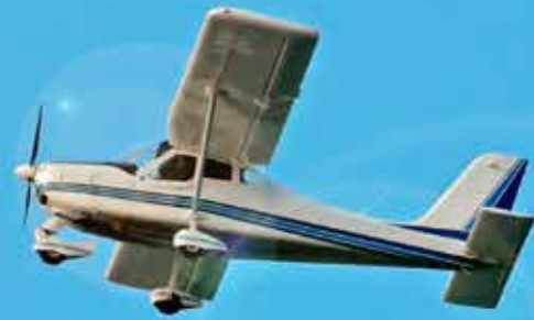
An advanced microlight, a Tecnam – about 600 kg, cruise 118 kt, stall 35 kt.
