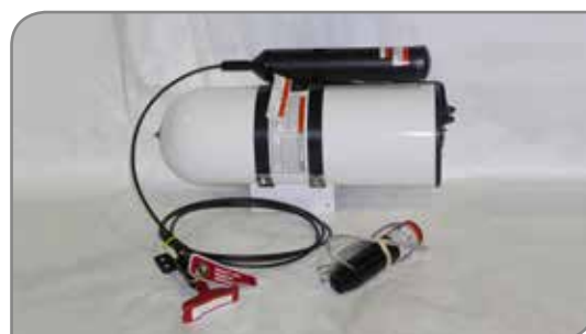
A complete ballistic recovery system showing the rocket (top), the canister holding the parachute, and the firing handle.
