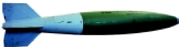
A 500-lb free-fall general purpose bombs used by Skyhawks for training exercises.
