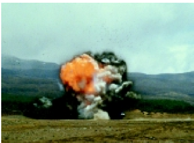
The destruction of a large quantity of obsolete ammunition in NZM301. Note the considerable amount of debris being accelerated vertically from the core of the explosion.
