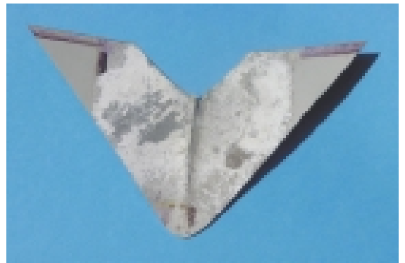
Severe internal rotor blade corrosion.
