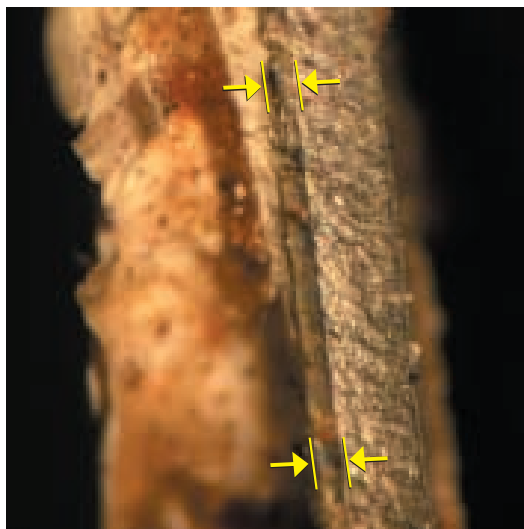
The bottom of the fin fracture on the starboard side showing the cut mark, as indicated by the arrows (at x 35 magnification).
