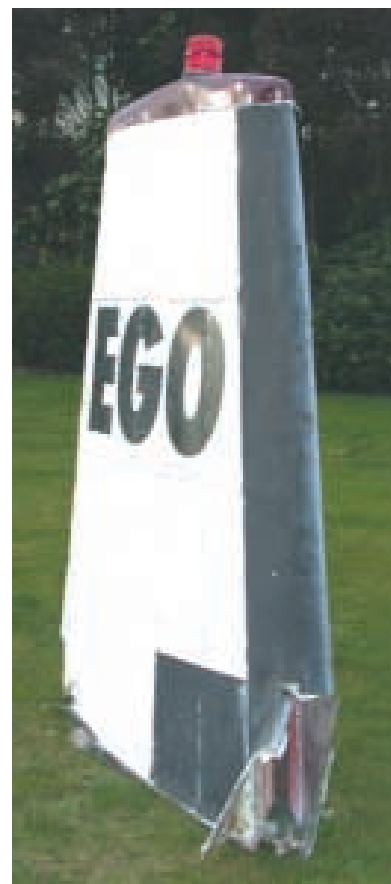
The failed tail fin.
