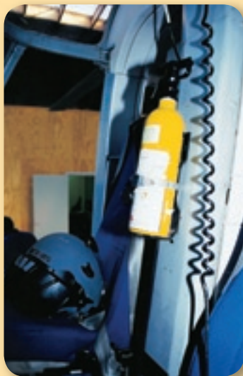
As yet, in New Zealand, there is no really good substitution available for halon (BCF) type portable fire extinguishers.
