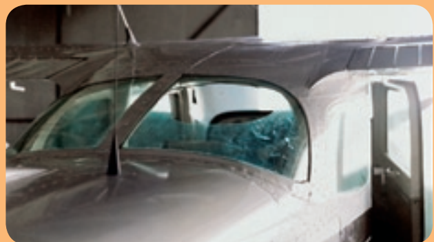
It has been known for the extinguisher to be expelled through the rear cabin window during aerobatics or in turbulence.
