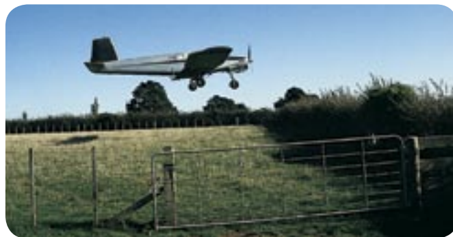
If possible remove the fence at either end of the strip or adjust the threshold accordingly.
