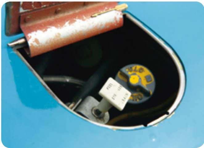
Fuel strainer drain on a C152.
