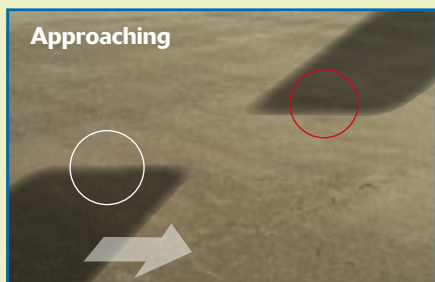
Glance at the shadows of the wings on the ground. If the shadows aren't going to touch, neither will the wings.
