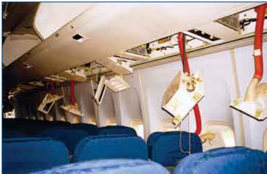
Three passengers were struck by overhead passenger service units that came loose in this relatively benign overrun accident. A good reason to get your head down early. Photo courtesy of Australian Transportation Safety Bureau.
