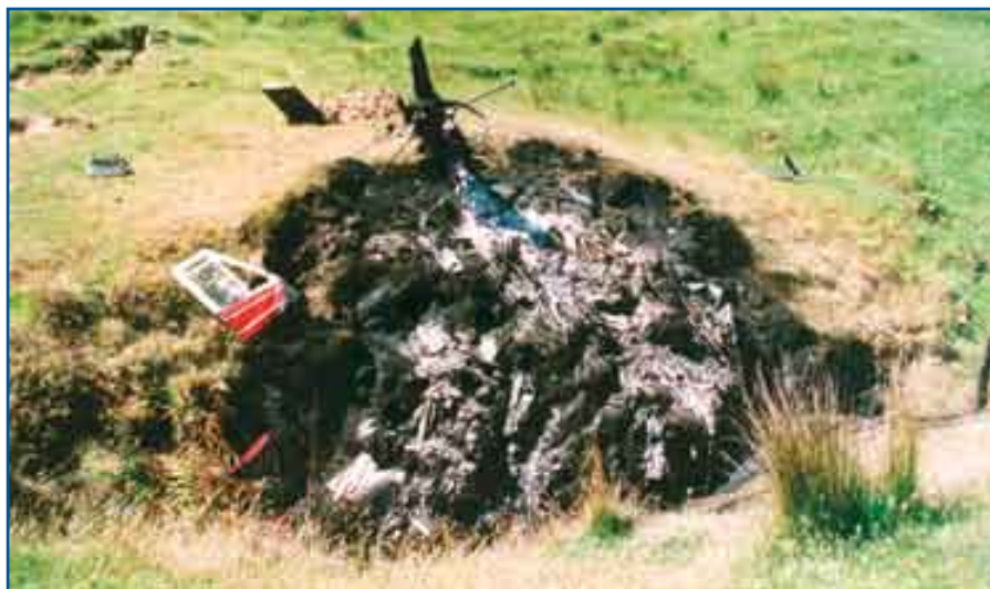
All that remained of a UH-1E helicopter after the main rotor was struck by the longline.
