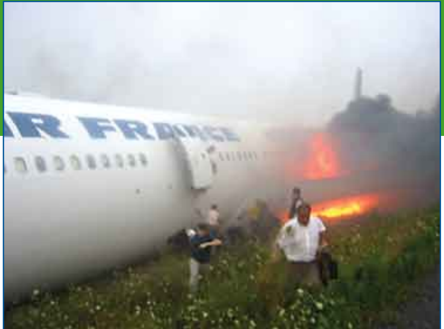
Passengers evacuating an Airbus A340 after an overrun at Toronto – note that the slide has not deployed. Photo courtesy of Transportation Safety Board of Canada.
