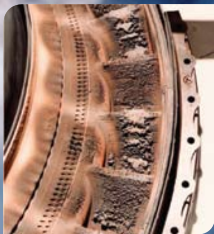
Damage to a turbine from a 747, flight BA009, in June 1982 in which all four engines failed. Photo courtesy of Captain Eric Moody.
