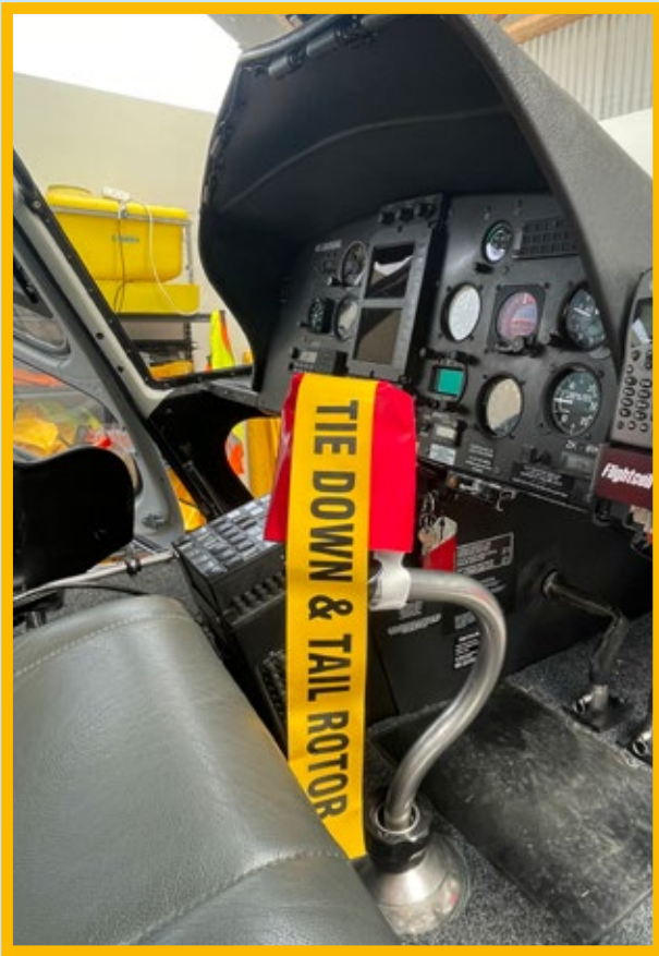
// Southern Lakes Helicopters have designed and made a 'witness indicator' which is placed on top of the cyclic.
