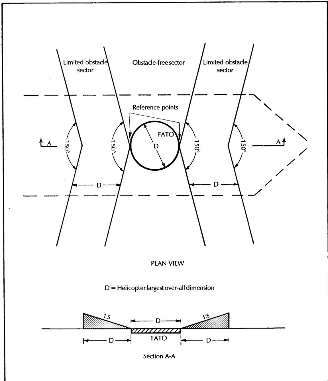
Figure 4-3. Midship non-purposed built heliport obstacle limitation surfaces
