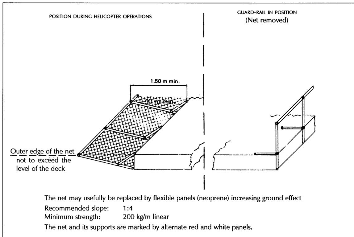
Figure 3-1. Collapsible guard-rail with movable safety net
