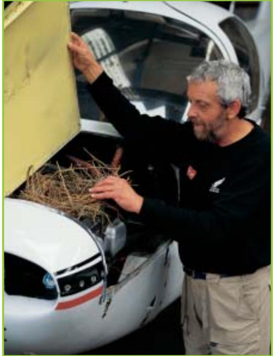
fire, the consequences of which need no further elaboration. Similarly, a bird's nest that disrupts the airflow into the engine oil cooler will almost certainly cause the engine to overheat and possibly seize. Nests built in the fuselage or wing can foul the control cables and could result in a control surface jamming.
