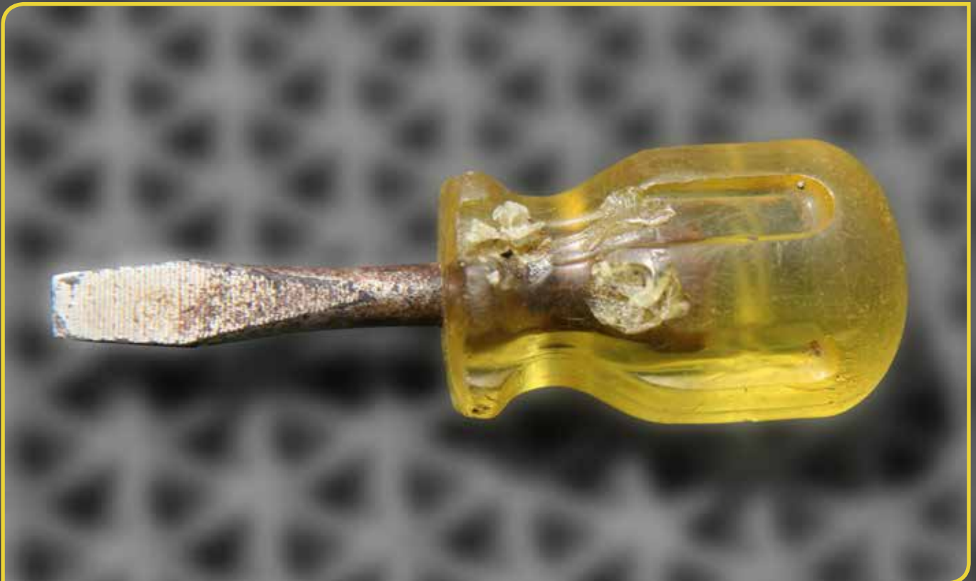
Safety investigators looking into a fatal crash in 2012 concluded that this screwdriver had remained in the rear-most section of the fuselage for some time.
