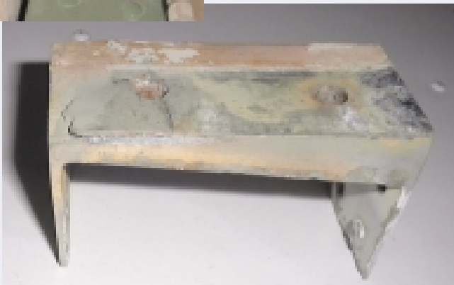
The offending wing/fuselage attachment prior to its replacement.
