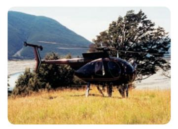
What factors should be considered when making a departure from a mountain pad? An adequate power margin at the hover is essential. As long as altitude can be traded for airspeed, takeoffs from pinnacles, ridgelines or other sites with clear areas below, offer the fewest problems.
