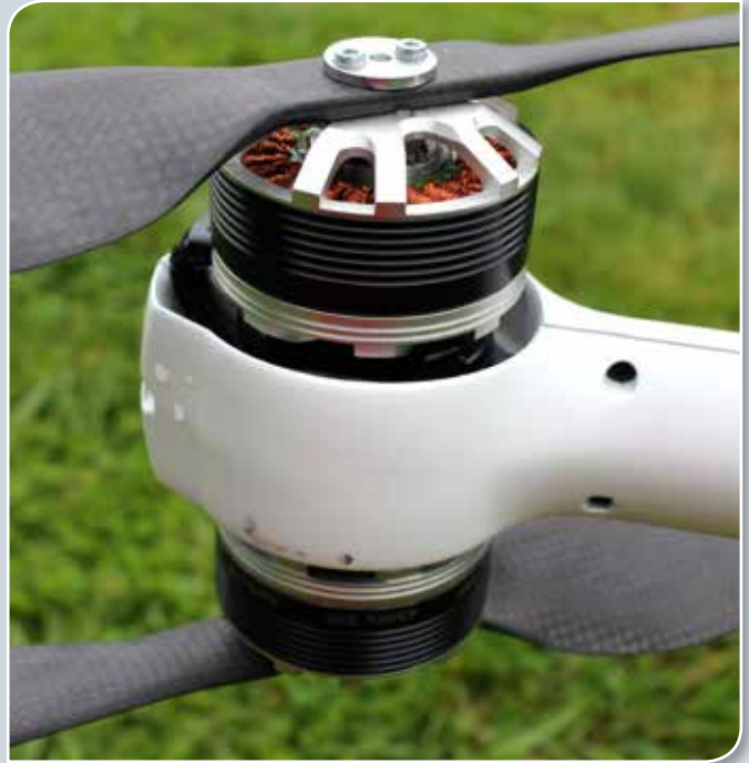
The coaxial propulsion arrangement on the SkyJibX4.
