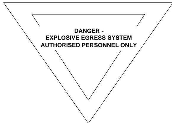
**Figure 1. Placard for egress system equipped aircraft**
