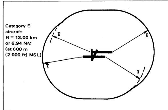
Figure III-8-1. Construction of visual manoeuvring (circling) area
