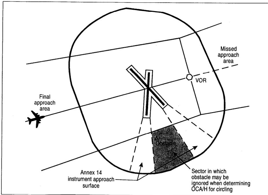
Figure III-8-3. Visual manoeuvring (circling) area — obstacle clearance
