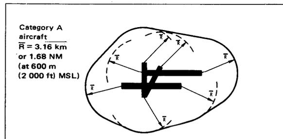
Figure III-8-2. Visual manoeuvring (circling) area
