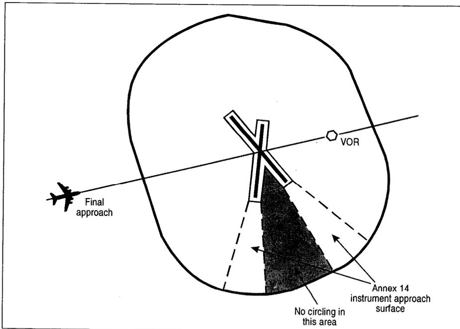
Figure III-8-4. Visual manoeuvring (circling) area — prohibition on circling
