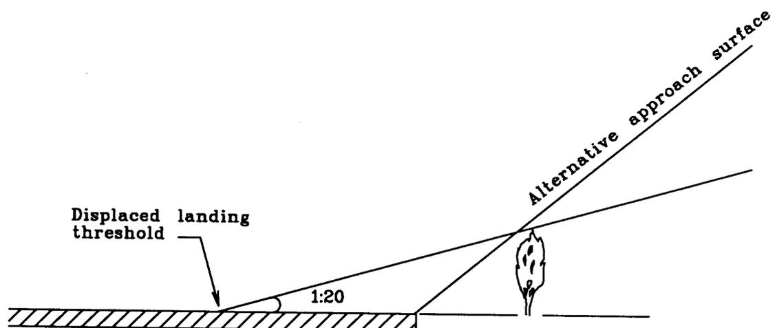
Figure 6. Approach surface obstruction clearance
