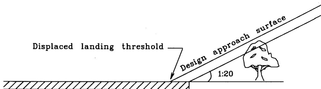
Figure 5. Aerodrome design approach surface - obstruction
