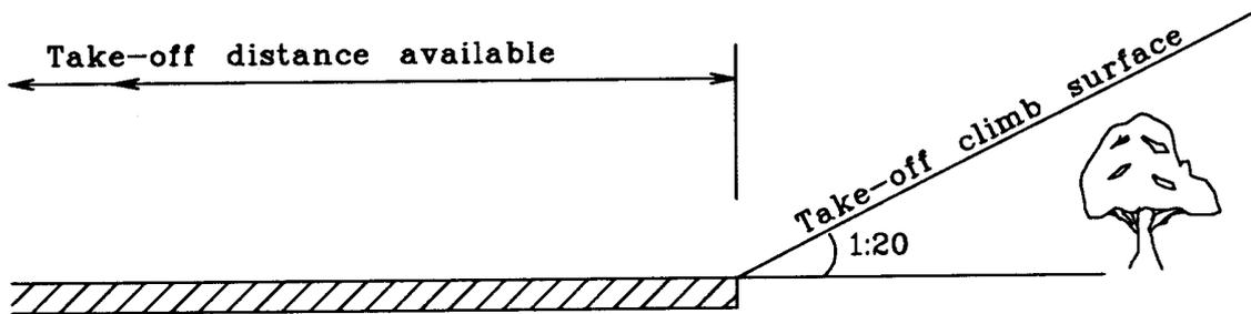
Figure 1. Obstacle free design take-off surface
