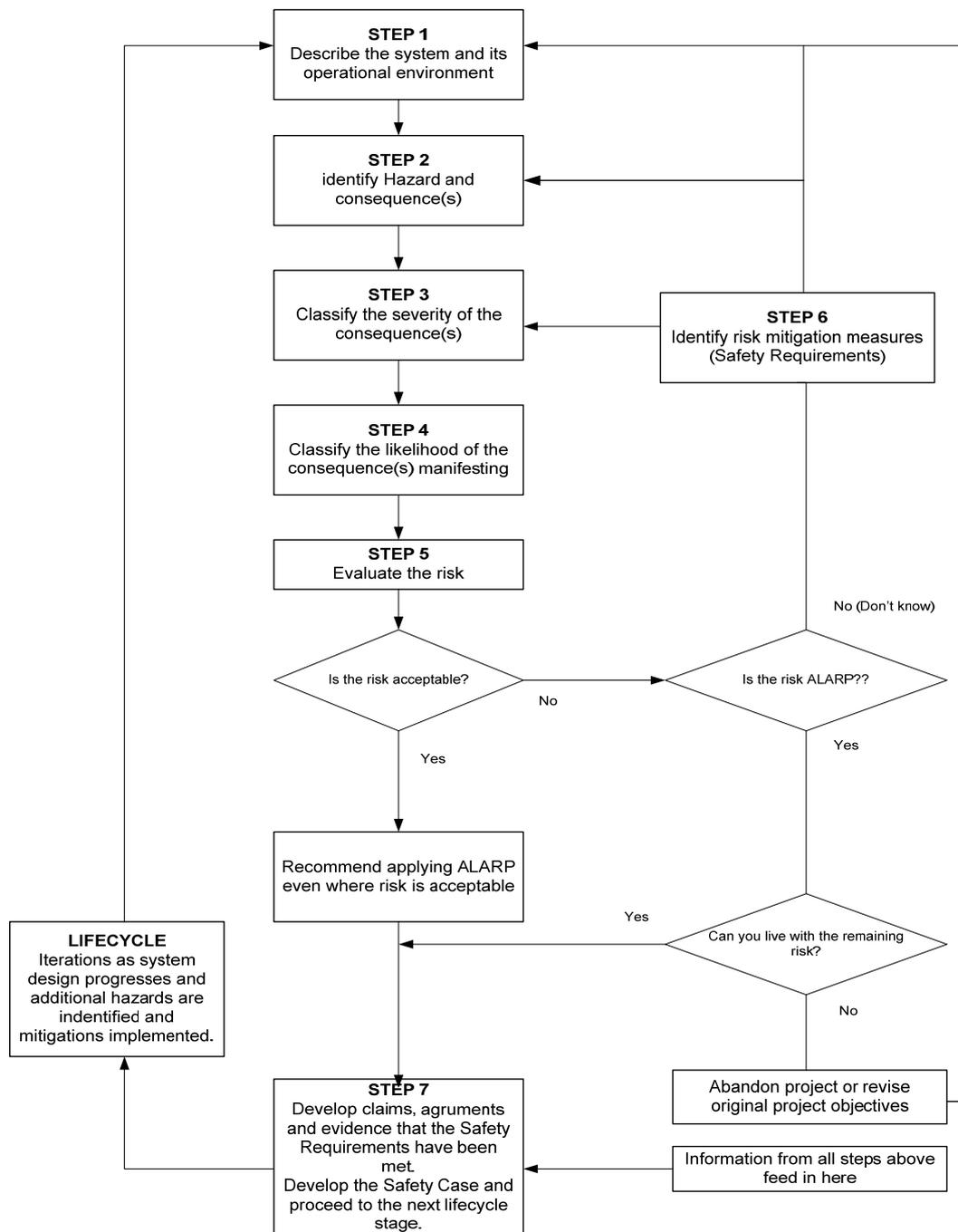
Figure 3: The Seven Step Approach (CAP 760 Chap 2)
