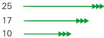
Wind gradient is the gradual decrease of the wind speed near the ground, due to surface friction and the air's viscosity. Discuss the effect it can have on the flare, in particular the inability to touch down at the planned point.
