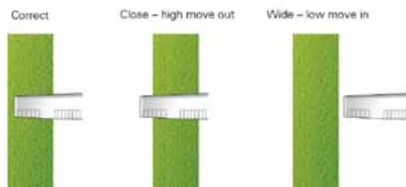
**Caption:** An example of how spacing is assessed using the parallel markings on a low wing aeroplane.
