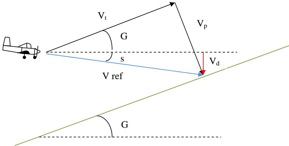
G = slope of the ground relative to horizontal.      s = aircrafts glide slope, below horizontal
