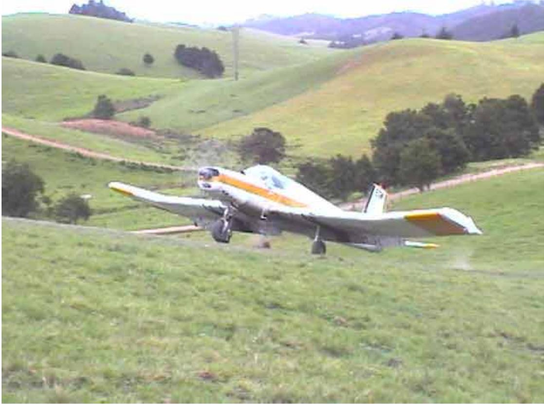
**Figure 3:** FU24 performing an uphill landing, note dirt flying up at point of impact.
