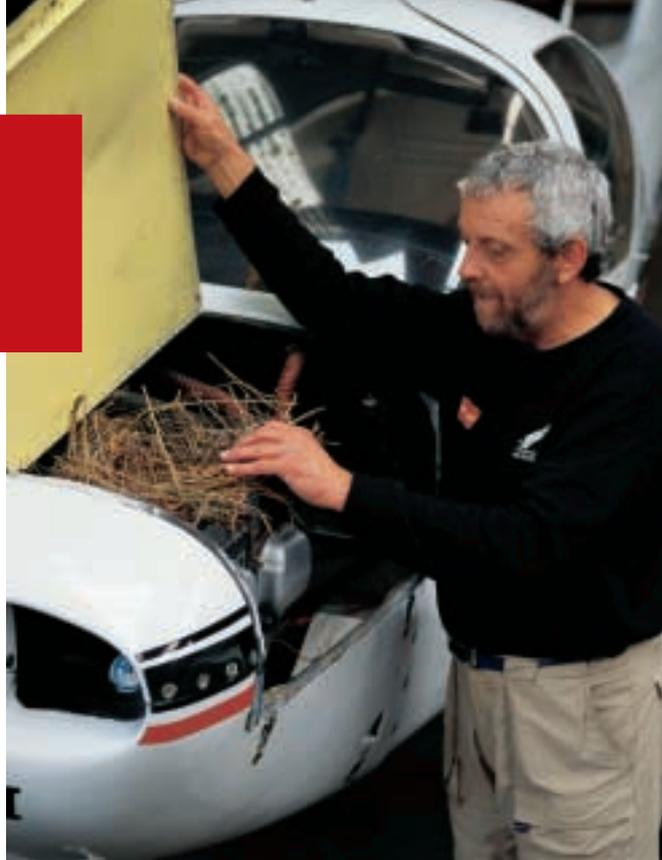
A careful and thorough inspection is required if aircraft have not been used for a while.
