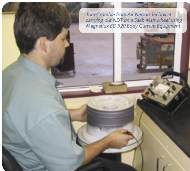
Tom Crombie from Air Nelson Technical carrying out NDT on a Saab Mainwheel using Magnaflux ED 520 Eddy Current Equipment.
