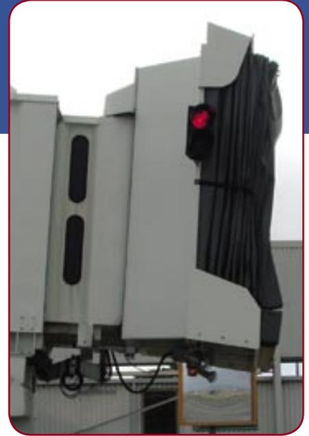
*The red light on the airbridge means it is unsafe for aircraft to dock.*
