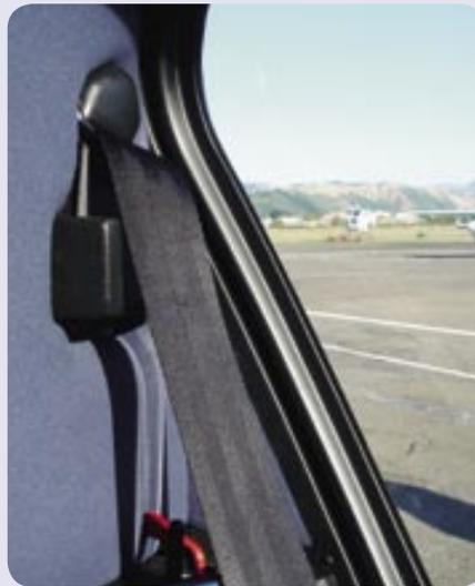
*Webbing must be in good condition and belts must retract properly like this example.*
