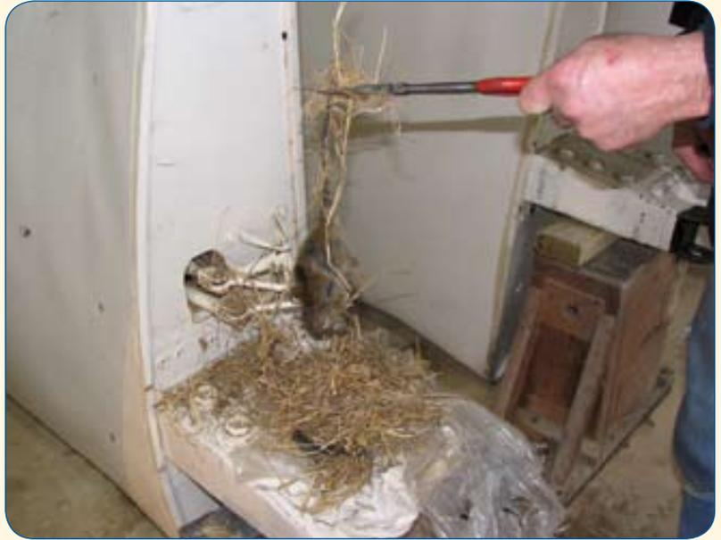
*Dead rats and nesting material being extracted from one of Gliding Hutt Valley's aircraft. This pile of foreign material would have been a serious threat to flight safety if left undiscovered.*
