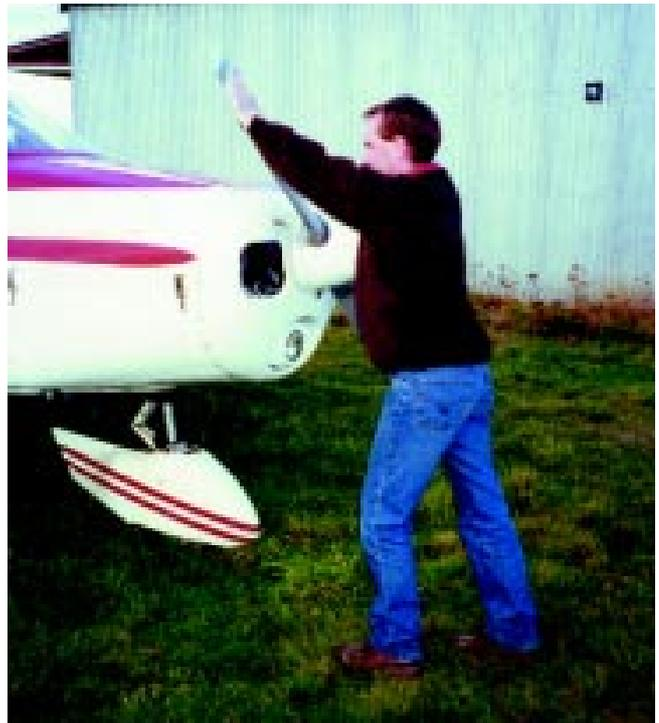
With a Gipsy engine such as on a Tiger Moth (rotating clockwise when viewed from the front) weight is transferred from the right to left foot and the prop-slinger walks away to the left (as pictured below).
