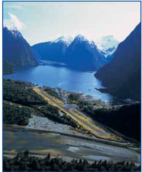
The constraints of surrounding terrain may dictate non-standard approach patterns but may also influence conditions of windshear, crosswind, sink, lift, etc.
