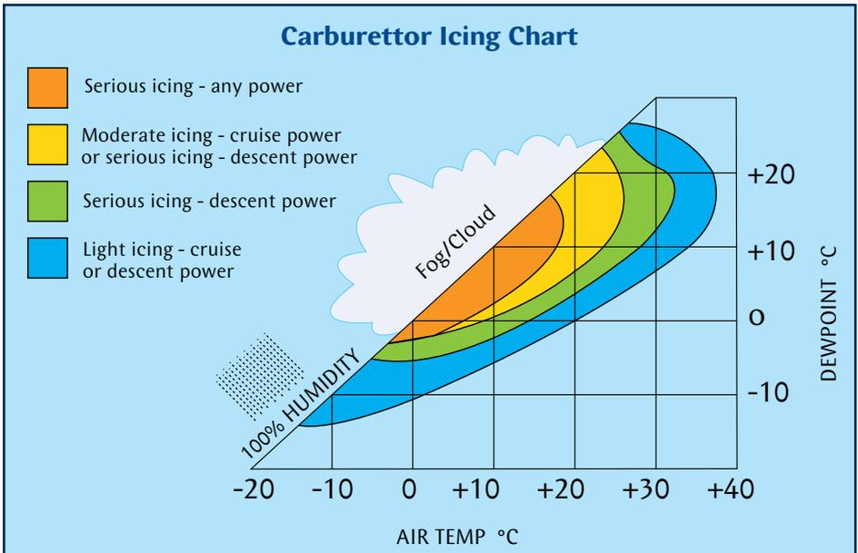
Alternate air should be selected until the aircraft descends into warmer air and the accumulated impact ice melts away from the engine air intake(s).
