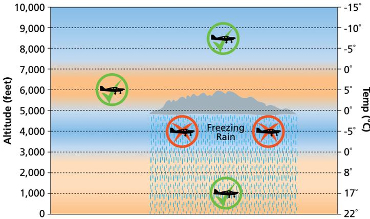
*This shows how a temperature inversion at altitude can produce conditions conducive to freezing rain.*
