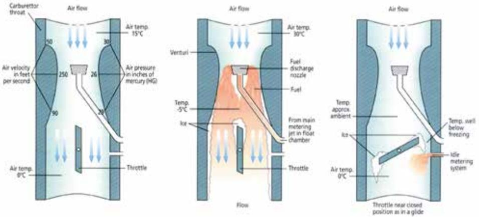
*Simplified views of a venturi showing changes in air velocity and temperature. These vary in relation to changes in throttle opening and engine rpm.*
